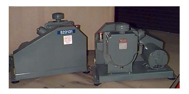
These are Welch Vacuum pumps. The items pictured are the same units with two views. As you can see there is a pump and electric motor mounted on a pedestal. The pump is driven by two belts. The size of the pumps are dependent upon the amount of vacuum required for the application.
