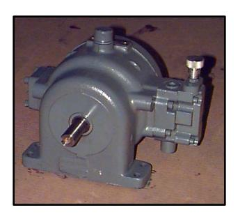
This is a PSV, 50 design, Racine / Bosch hydraulic pump. This is a compensated, vane type pump. It is subplate mounted. These pumps come in various styles and flow sizes. These can be from 10 GPM to 25 GPM in this basic style.
