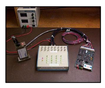
K+S Services Inc. would like to announce full power dynamic testing for the Data Logic HS870 Series Programmable Controller. The test system is capable of fully exercising all inputs, outputs, communication, and antenna functions.
